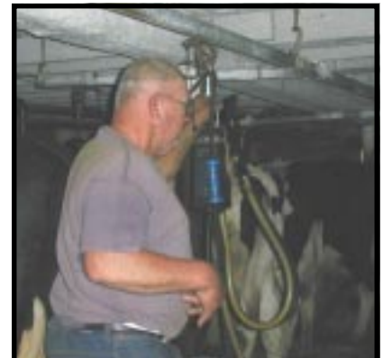
Maurer using the monorail track for moving milking units between cows. Photo courtesy AgrAbility for Pennsylvanians.
