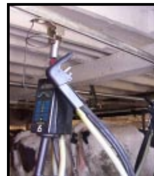
DeLaval’s one-handed snap-on connection cluster for electricity and vacuum makes milking easier for Maurer.
