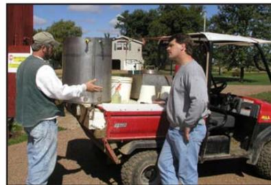
*Purvis explains how an old water heater he mounted to the Kawasaki Mule makes for easy hauling of water and milk replacer to the calf hutches.*
