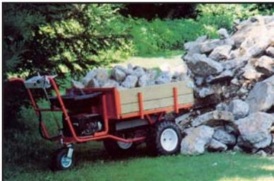
Using a powered wheelbarrow, such as the DR Powerwagon from Country Home Products, may reduce back strain associated with carrying heavy loads.
